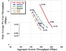
Figure 2. Edge TATP Vs ATP for (30,50,70) users/cell with 3Mbps/user.
